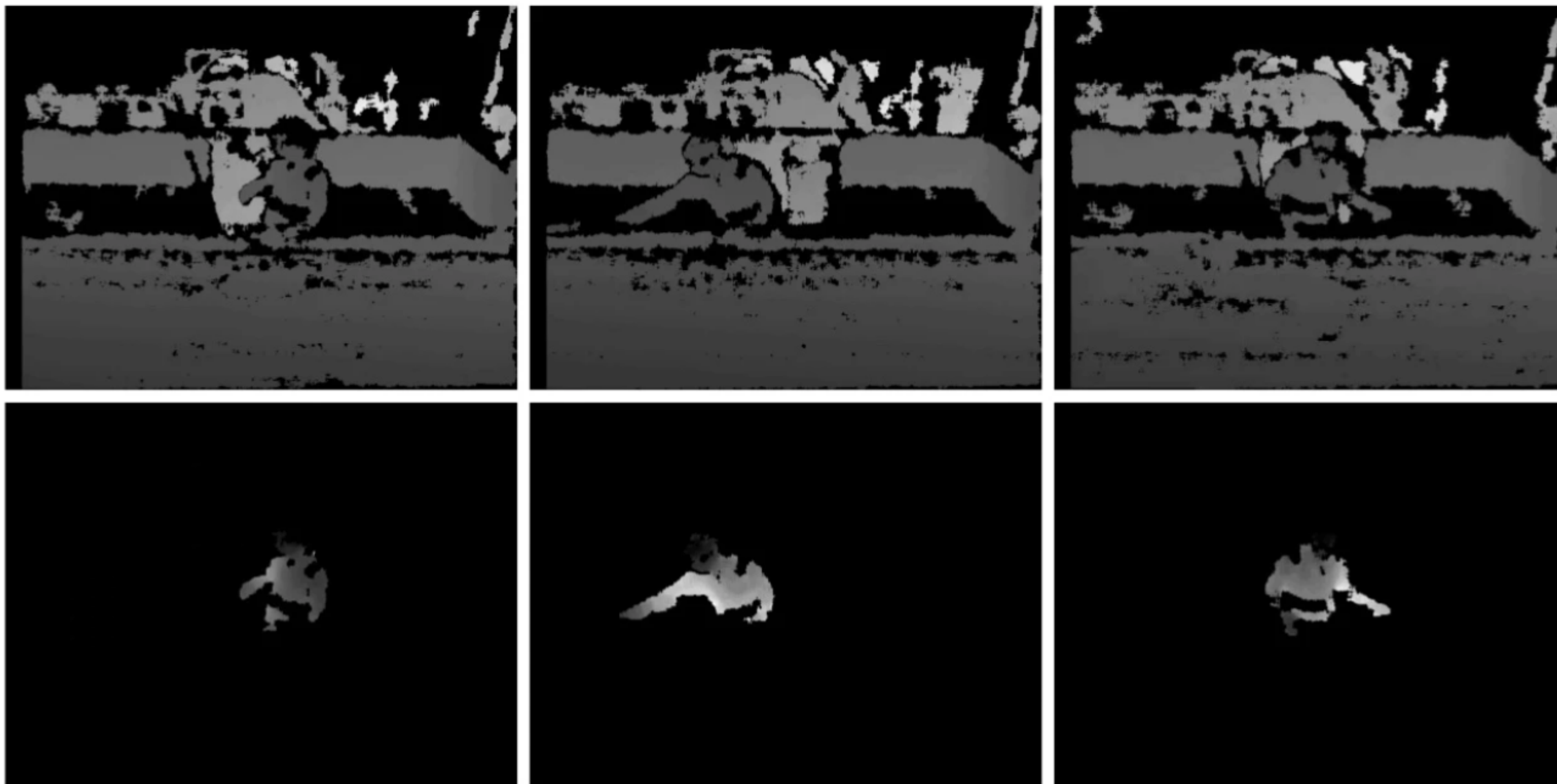
Raw depth frames (top) and segmented depth frames (bottom)
